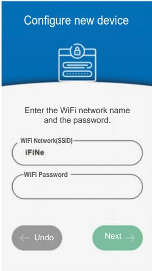
Once you have entered the device configuration mode, you will be asked for the credentials of the Wi-Fi network on which the device will be connected (network name and password).
